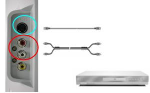
the other end to the audio connectors associated with the AV1 input on the side of the HDTV.
